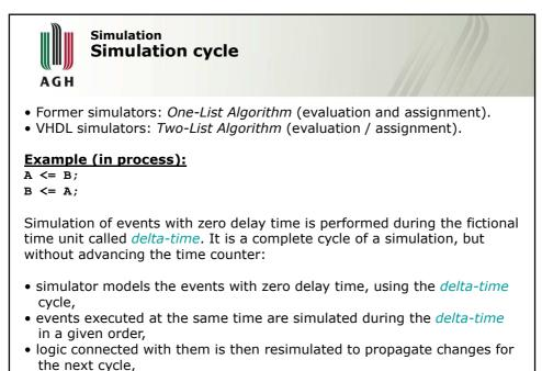
• delta-time cycles are repeated until no changes are detected.
